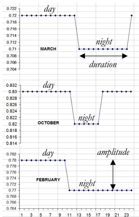
The interesting thing appears to be the fact the amplitude of movement doesn't change significantly over a typical season, but the length of the signal extends in the colder months. Buildings naturally take longer to warm up following cold nights.
