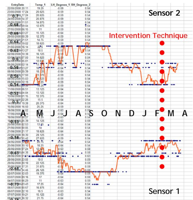
The red lines plots a 6 Interval Moving Average used to reduce signal fluctuations
