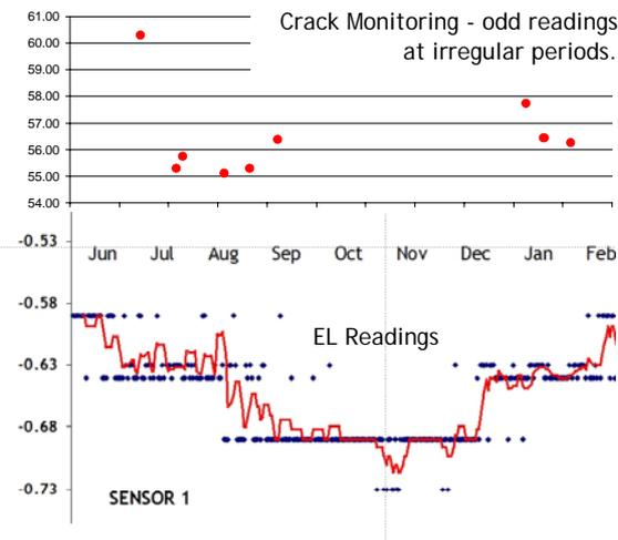
Crack monitoring (upper of the two graphs) tells us there is enhanced periodic movement that implicates the tree, but we can hardly take comfort in delivering this level of service when an alternative technology, costing little more, delivering objective data at regular intervals, is available.
