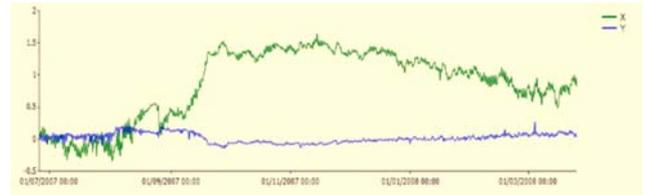
Readings were taken every 8 hours, day and night, and sent direct to the web portal. We can see clearly the periodic signature implicating a nearby tree. In addition we detect diurnal movement - around 0.2mm on the 6<sup>th</sup> March.
